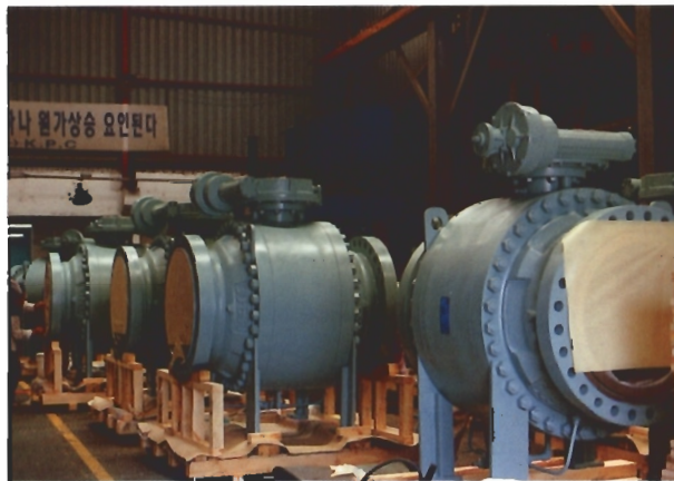
3 PIECE TRUNNION MOUNTED BALL VALVES, SIZE 2" UPTO 42", CLASS 150 UPTO 1500.
