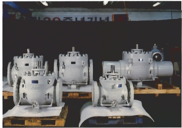
TRUNNION MOUNTED TOP ENTRY BALL VALVES, SIZE 2" UPTO 30", CLASS 150 UPTO 2500.
