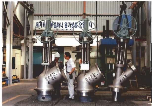
SPECIAL ANGLE VALVES, SIZE 1" UPTO 30", CLASS 150 UPTO 1500.
